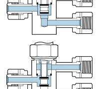
When there is no pressure to the actuator, the stem tip seals the lower port, allowing flow through the upper port.
